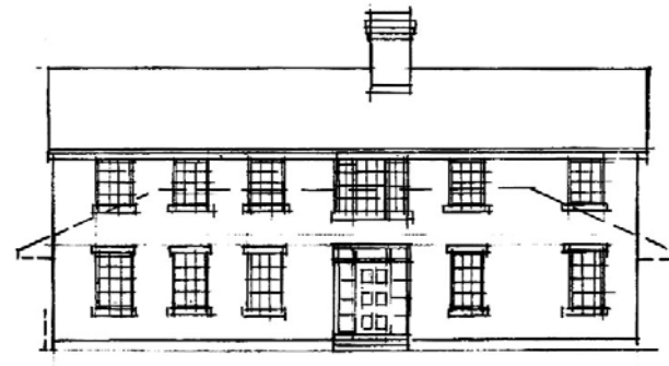
The Historical Conversion approach used in putting a second storey addition on the same house above
